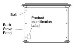
Figure 6 - Removing Back Panel
